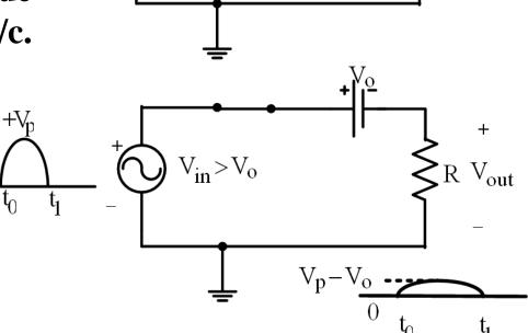
If  $V_{in} < V_o$ , then current will be flowing from the cathode to the anode. Hence, diode is rb. Diode is represented by an o/c. Current is 0.  $V_{out} = 0$ .
