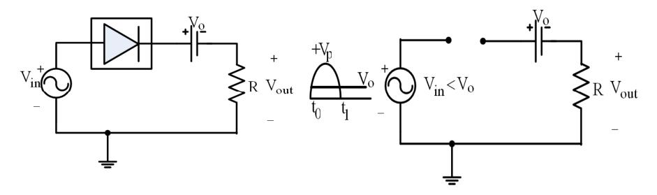
• Diode fb (ON),  $V_{out} = V_{in} - V_o$ . If  $V_{in} = V_p$ ,  $V_{out} = V_p - V_o$
